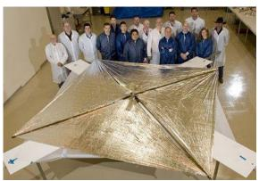
**Fig [3]:** The prototype sail in front of NASA team on Solar Electric Propulsion, courtesy-NASA. Various program goal have been attained, including certifying solar radiation pressure (SRP) issues on the sail and performing in-flight supervision and navigation approach using the solar.
